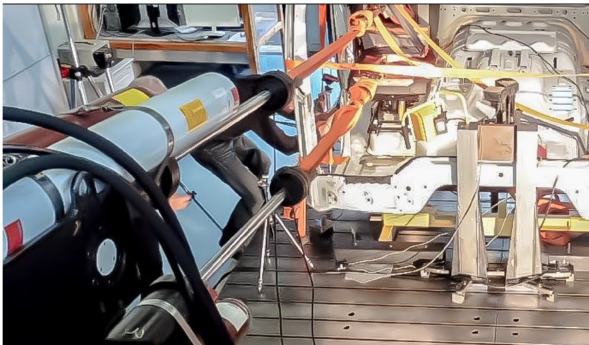
Volvo Group Europe performs the ECE R14 seat belt anchorage test on the composite seat reinforcement plate, which is attached to a truck cabin. The seat was loaded with a total of 80 kilograms across the seat's shoulder and lap section while cables connected to an actuator pulled the weights forward in the cab. Photo Credit: Volvo Group Europe
