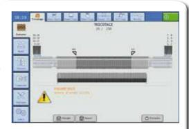
The new 12" color LCD screen gives the operator the possibility to interact with the machine, to access directly to the desired functions and to intervene simply and rapidly.
